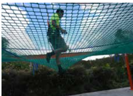
Dynamic load testing of Safety Nets.
