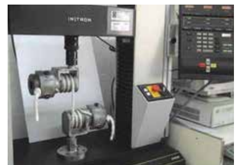
Laboratory Testing of Ropes and Net cords
